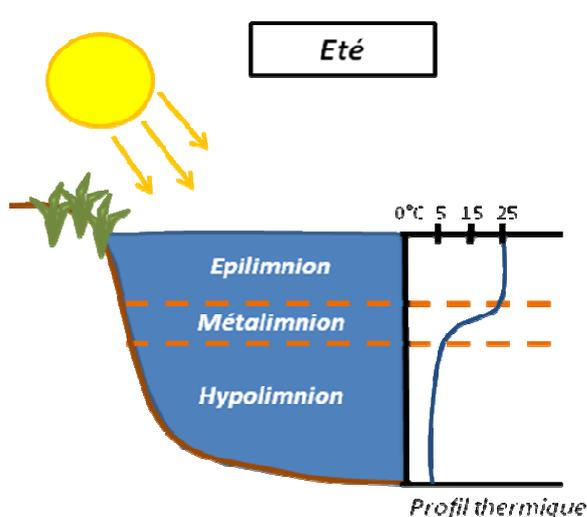
Figure 6 : Stratification installée
